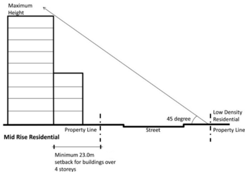
Figure 10.15b: Application of 45 Degree Angular Plane
