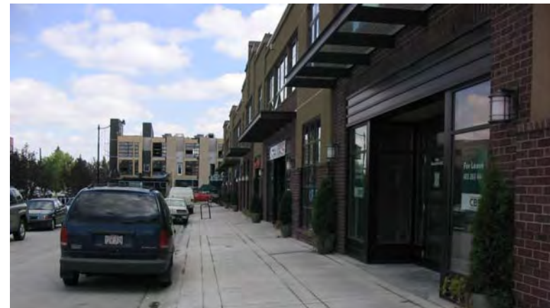
Building entrances are located at intervals of every 6.0 - 8.0 m along the building façade. The entrances are highlighted through the use of accent materials, planting, canopies, and architectural lighting.
