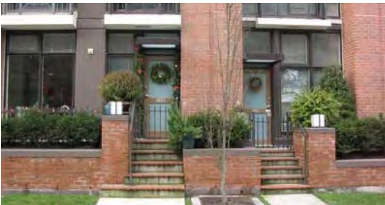
Individual entrances into residential units on the ground floor are set back 3.0 m from the property line and are raised 1.0 m above the street level to accommodate landscaping and maintain “eyes on the street”.
