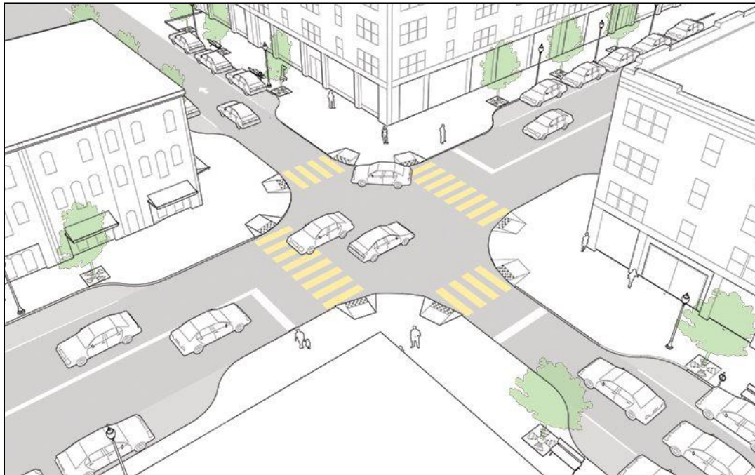
Figure 8.19: Shorter Pedestrian Crossing Distances using Corner Bulbs, from NACTO's Urban Street Design Guide
