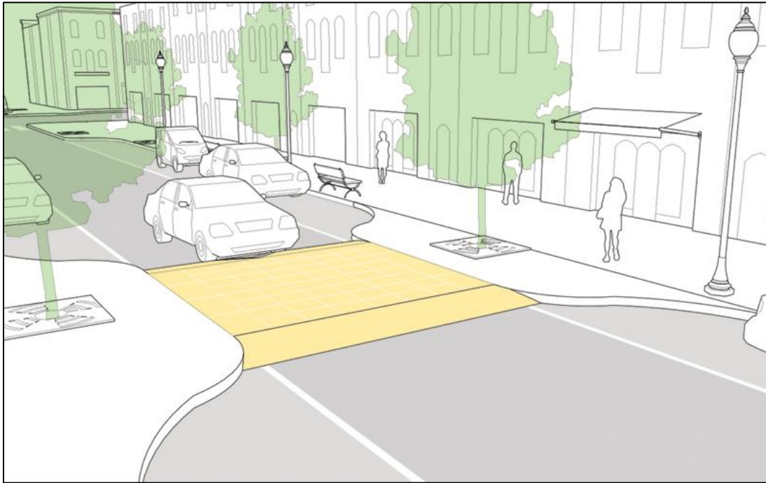
Figure 8.8: Vertical Speed Control Element – a speed table from NACTO's Urban Street Design Guide Speed cushions are speed humps or speed tables that allow emergency vehicles or buses to traverse the hump or table without a vertical deflection (see Figure 8.9).
