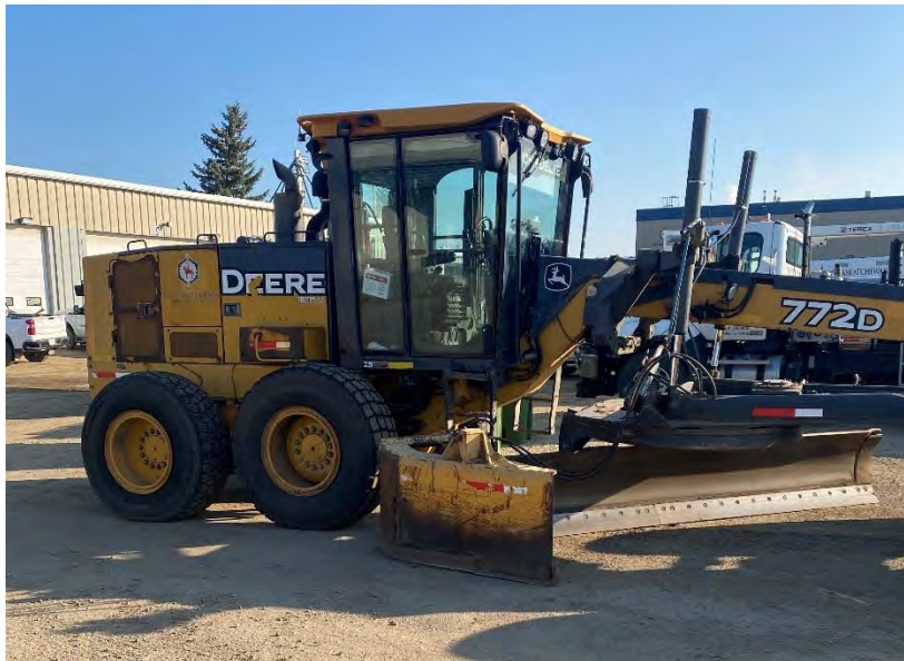
Grader with Gate (used during residential snow clearing to avoid windrows on driveways and entrances)
